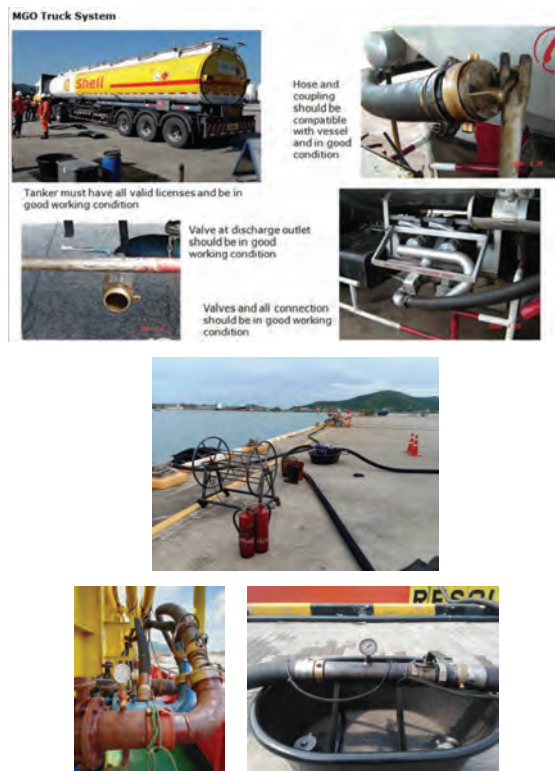
Installation Pressure Gauge at Truck side & Ship side
